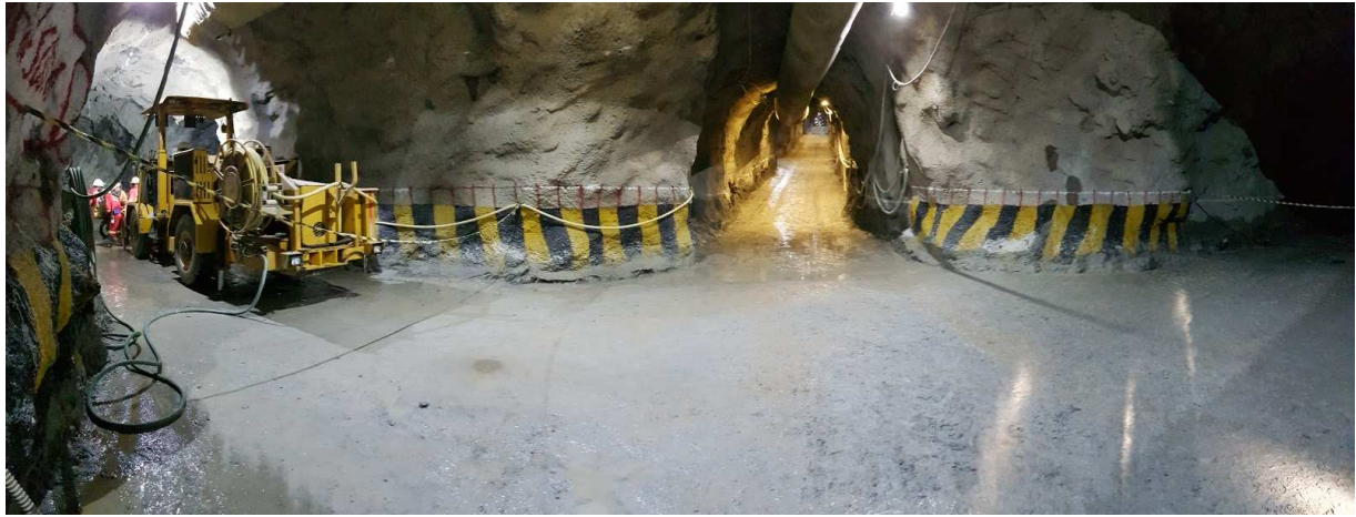
Footwall drives intersecting the main decline
